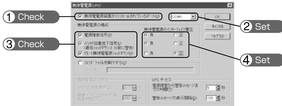
Set each signal interface voltage setting as shown below.
